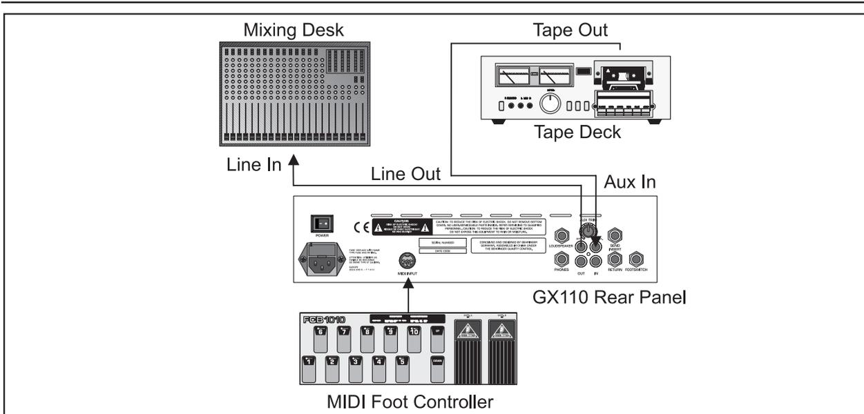
Fig. 2.2: Expanded setup
